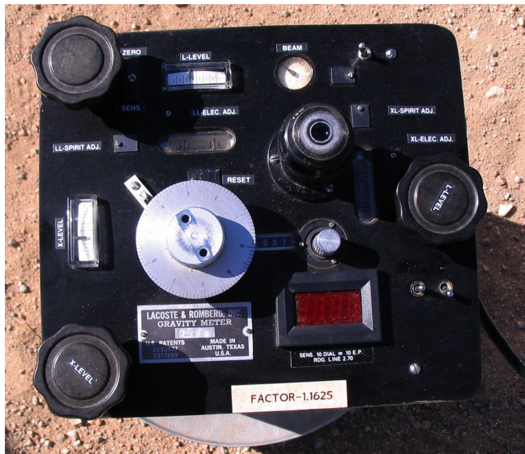
Figure 9 Top view of LaCoste and Romberg D gravity meter. Tilt adjustment knobs are located on the left and middle right. Galvanometer dial is above the eyepiece and the aluminum read out dial is in the middle.
